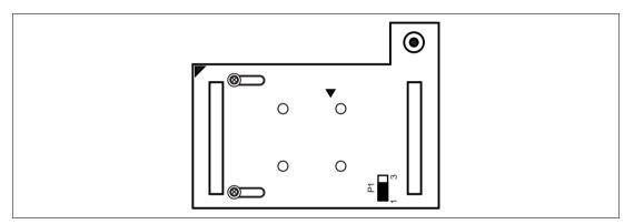
Figure 10 P1 Jumper Socket
